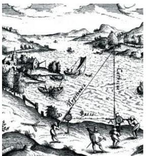
Measuring the width of a river by triangulation
